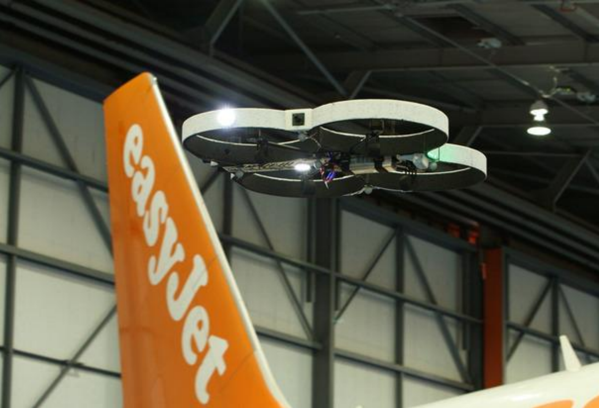
UAV used by EasyJet for fuselage inspections
